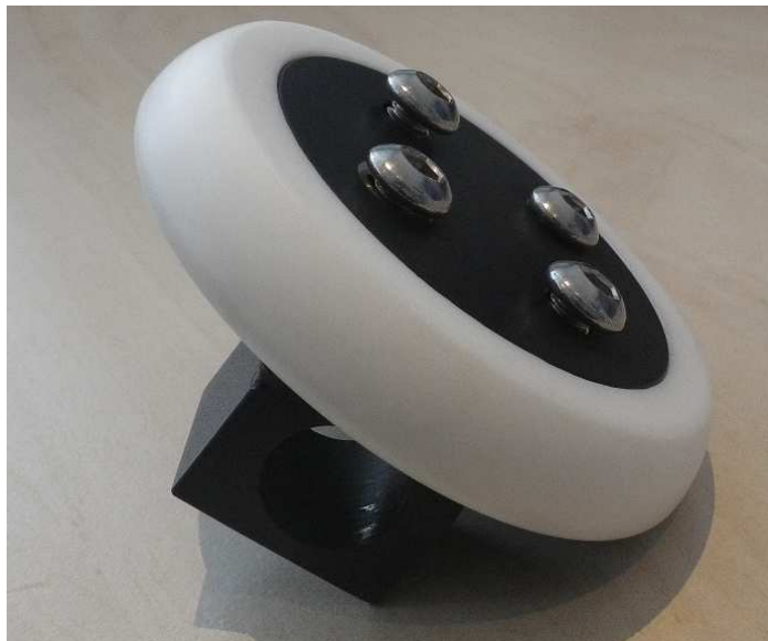
Figure 3: Butterfly with PTFE profile for low friction
